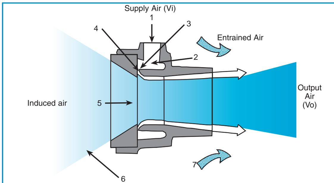
$V_i$  = Volume of supply air (free air at atmospheric pressure)
